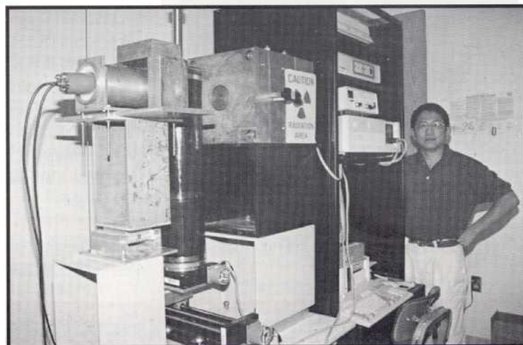
Hsuan-Tsung Hsieh, post doctoral fellow, stands beside the CT scanner used to study hydrological properties in rocks and soils.
